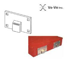
**Hook Section Connector** 3/16" plate with square holes for mounting with 5/16" bolts, (not included). Galvanized finish.
